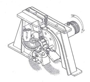
Before maintenance, shot blast machine and its moving parts should be made safe against running by mistake. This is possible by a lockable switch.
