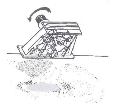
In order to detect "hot spot" of blasting area which is the center of biggest intensity of blasting, a thin metallic sheet which is placed in the position of work piece to be shot blasted. Length of metallic sheet should be minimum 1,2 m so that sheet should cover impact wall. Than a one minute blasting is done without changing the position of metallic sheet. (Rotation should be switched off) After removal of steel sheet, highly heated area "hot spot" should be noted against accidental burning.
