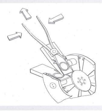
After removing of cover and armors, blades become accessible for replacement. For blast cabins in which access from inside of cabin is possible, replacement of blades is also possible from inside of cabin. Blades are removed by means of special pliers. After fixing springs removed, blades can be taken out of its conical placement.
