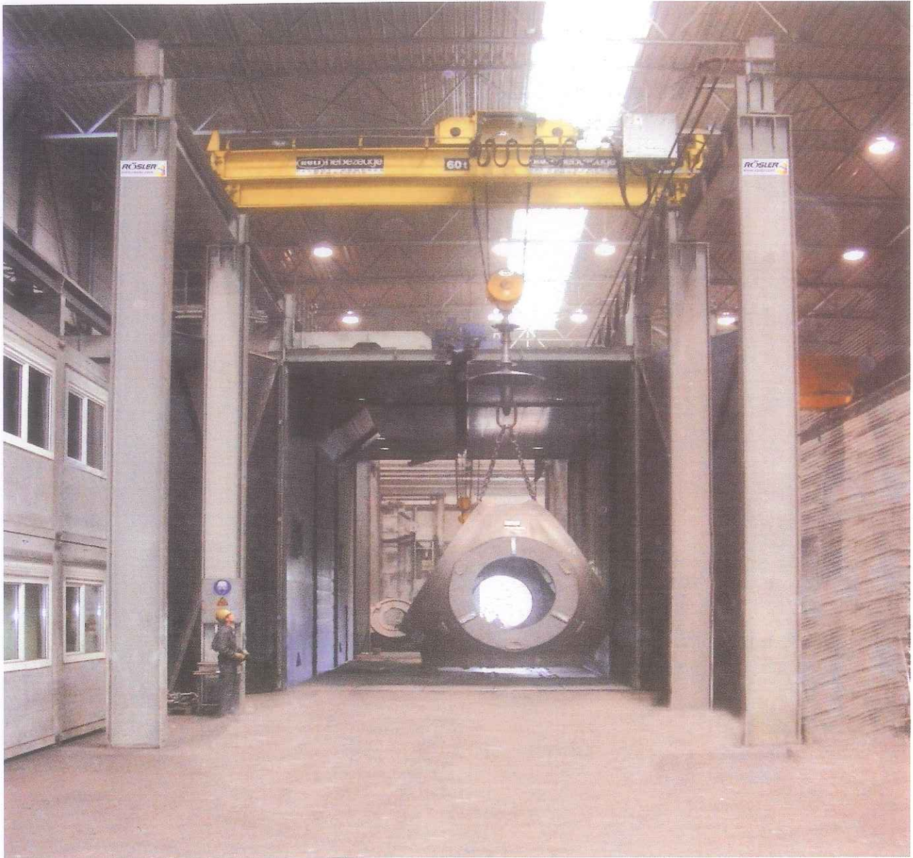
(Picture 1) Room type shot blast machine
